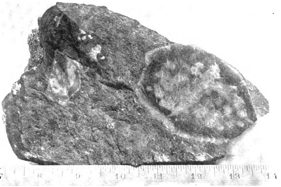
A. HAND SPECIMEN OF ANDESITIC BRECCIA WITH INCLUDED ACID FRAGMENTS. THE LIGHT COLORED STREAKS AND SPOTS IN THE FRAGMENTS ARE "ZONES OF GROWTH" FROM WHICH SMALL SPECKS OF IRON ORE HAVE EVIDENTLY DERIVED A PORTION OR ALL OF THEIR MATERIAL.
